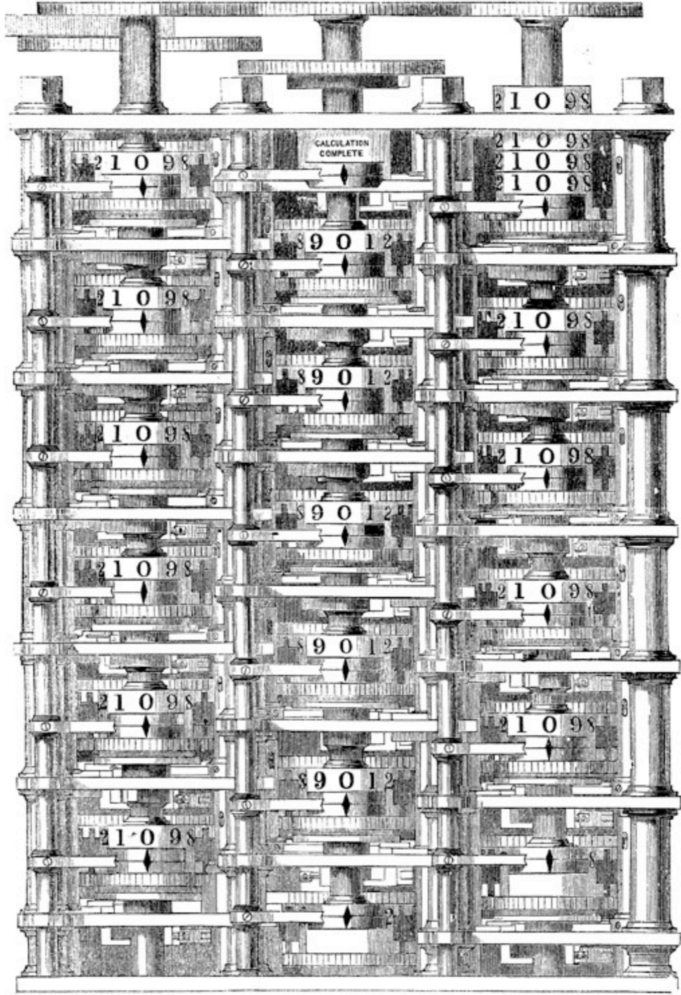
PORTION OF BABBAGE'S DIFFERENCE ENGINE.
