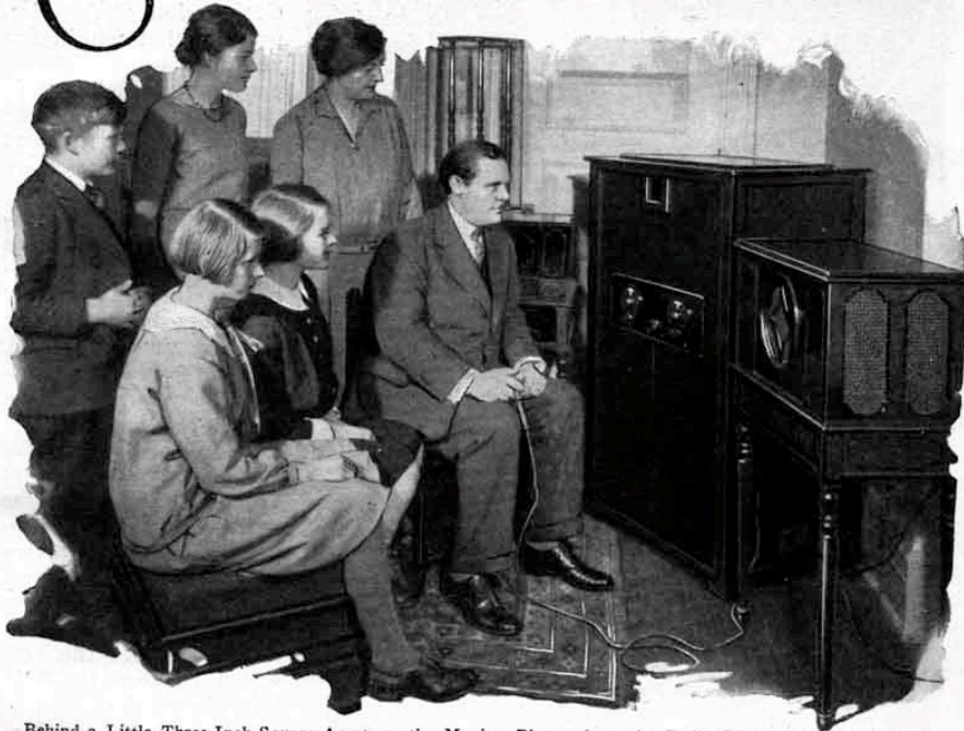
Behind a Little Three-Inch-Square Aperture, the Moving Picture from the Radio Studio Appears, While the Watcher, with a Push Button in His Hand, Keeps the Picture Synchronized
